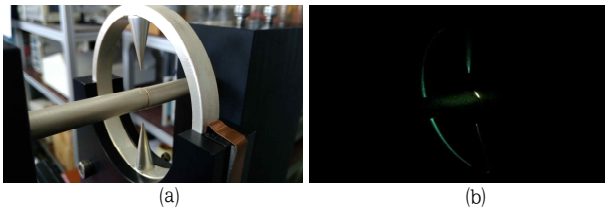
Fig. 7 An actual arc-induction type DC CB, (a) The fabricated arc induction needle, (b) The actual arc.
