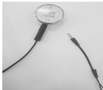
Fig. 6 Stethoscope Type Microphone Sensor
