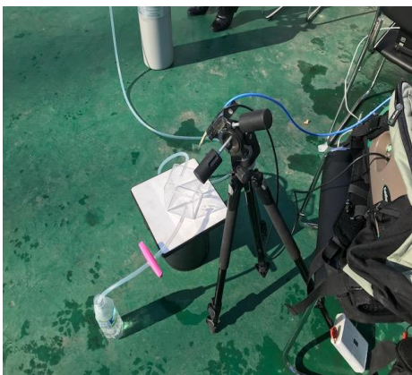
Fig. 3. Observation setting to measure spectra of NO 2 and SO 2 gases using a hyperspectral sensor
