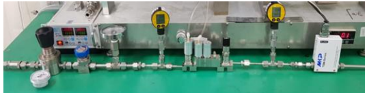
Fig. 9. Block Valve CV Test
