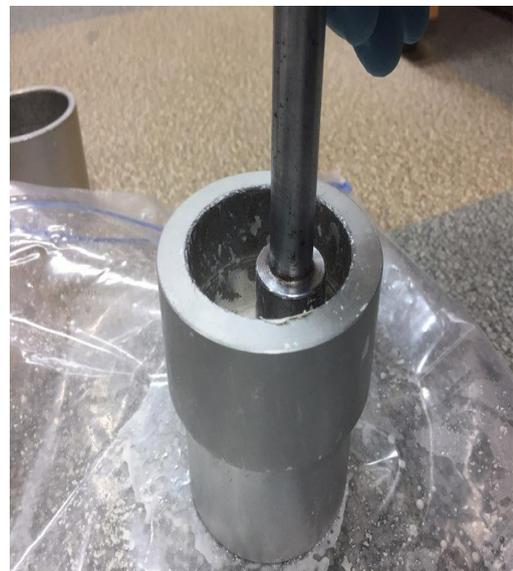
Fig. 4. Specimen cup and cap, rammer
