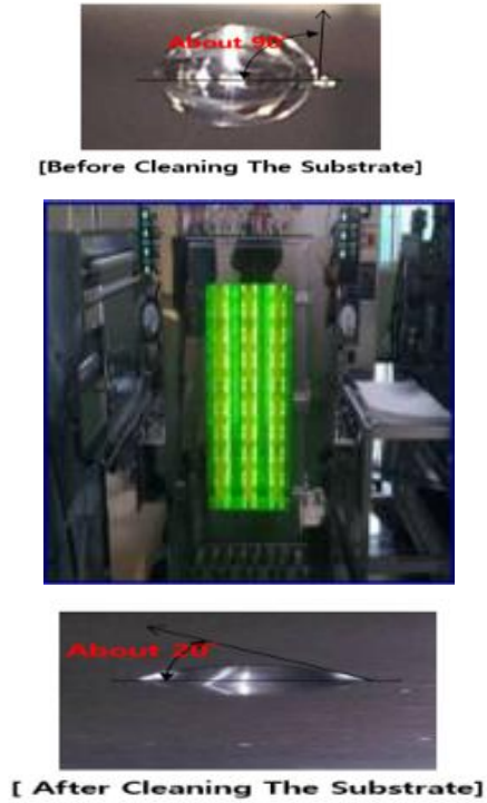
Fig. 5. The Anode Substrate UV Cleaning Results
