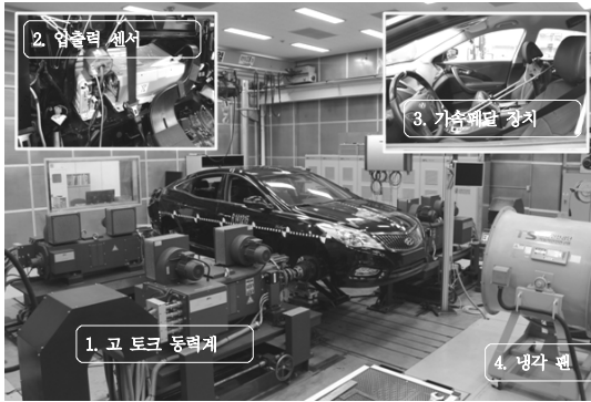
Fig. 1 Powertrain test bed with traction battery monitoring and accelerator control devices for hybrid electric vehicles
