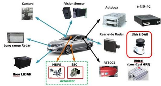
Fig. 1 Hardware configuration of the autonomous driving system
