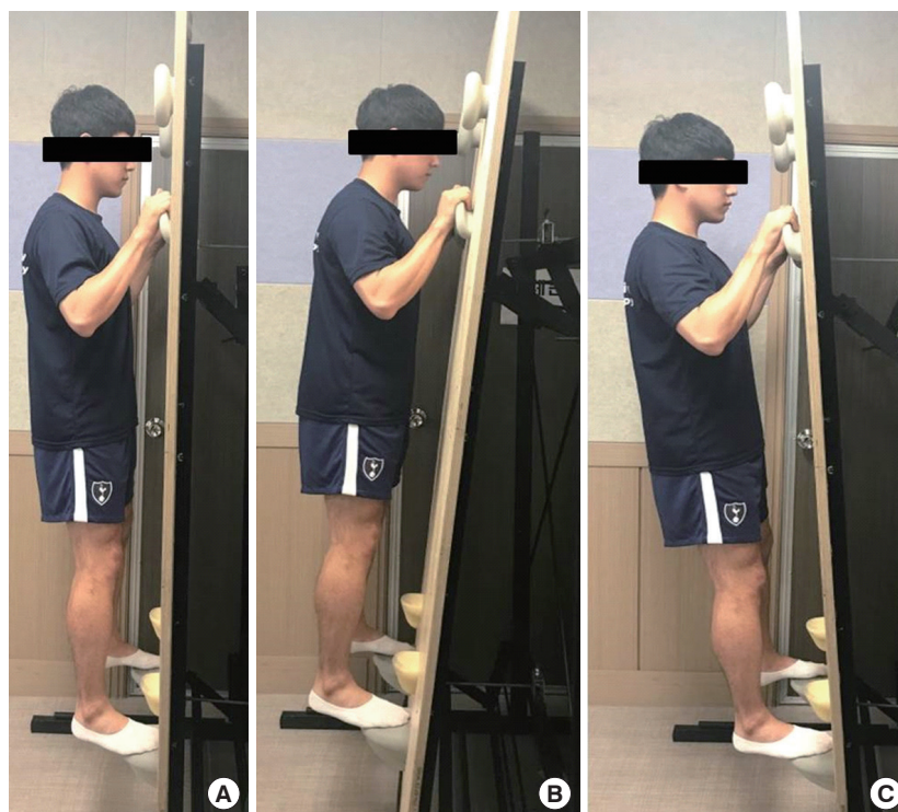
Figure 1. The climbing wall inclination angles (a. 0°, b. +15°, c. -15°).
