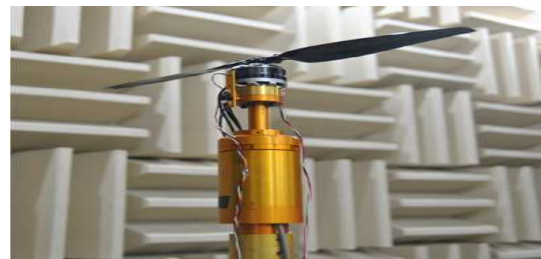
Fig. 6. Single-component testing device
