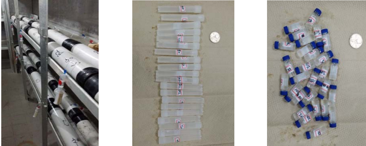
Fig. 4. Pore fluid sampling and pre-treatment for geochemical analyses.
