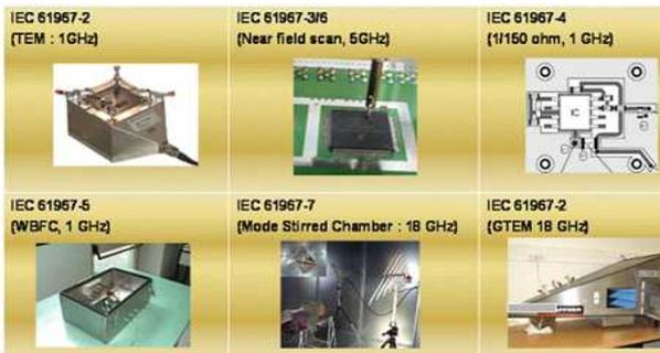
Fig. 1. IEC 61967 EMI measurement standard
