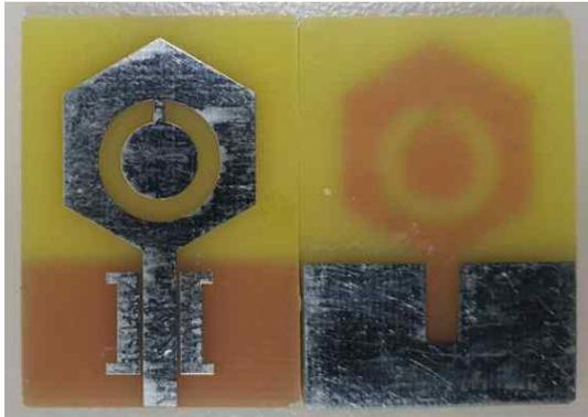
Fig. 2. Photo of the implemented antenna.
