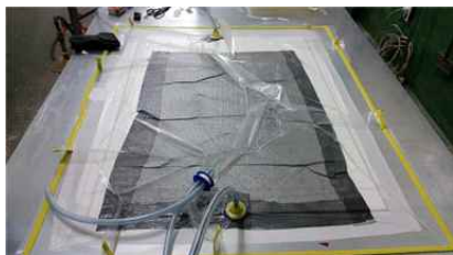
(a) 진공 상태 확인시험 (a) Test of a vacuum state
