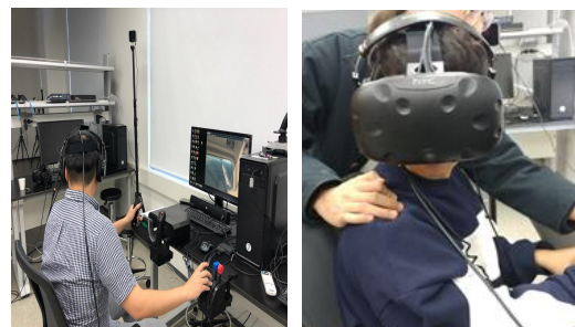
Fig 2. VR HMD based Basic Aviation Training Device
