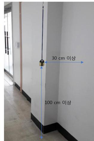
Fig. 1. Radon detector installation of learning space.
