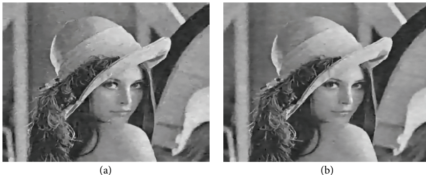
Fig. 2. Denoising result for Lena corrupted with a noise standard deviation \sigma = 30 . (a) EPLL PSNR = 30.66. (b) Proposed operator based on EPLL PSNR = 30.85.
