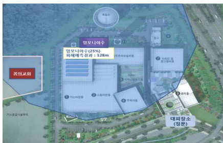
Fig. 8. Ammonia water leak maximum damage range
