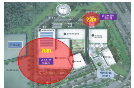
Fig. 7. NG Explosion maximum damage range
