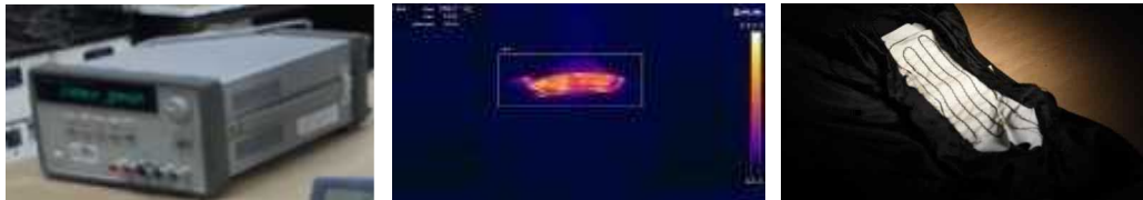
Connecting to 24V Infrared thermo-graph image Trace of a burning of the hot wire
