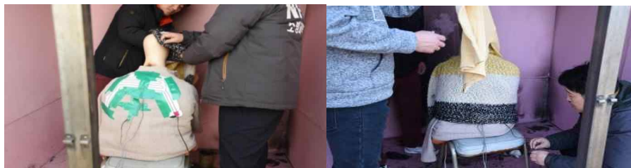
Fig. 7. Combustion experiment of 12V electrically heated jacket with wool and nylon sweater.
