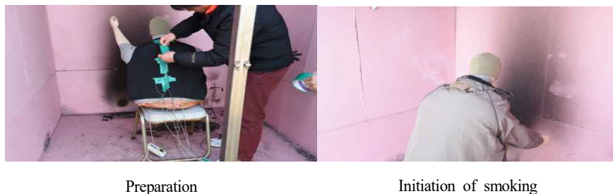
Fig. 5. Combustion experiment of 12V electrically heated jacket with polyester coat.
