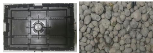
Figure 3. Figure of vegetation unit and artificial soil
