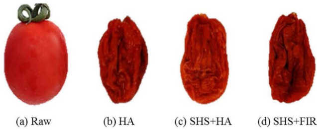
Fig. 1. Appearance of dried cherry tomato. (a) raw tomato, (b) HA; hot-air drying, (c) SHS+HA; superheated steam combined with hot-air drying, (d) SHS+FIR; superheated steam combined with far infrared drying.
