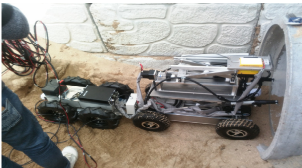
Fig. 6. GPR device in sewer
