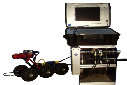
Fig. 2. Exploration device used in the sewer
