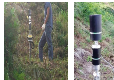
Fig. 13. Installation takes less than 30 minutes for one Guerrilla sensor
