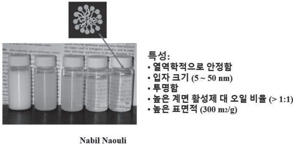
Fig. 3. Physicochemical properties of microemulsion (Naouli et al., 2011).
