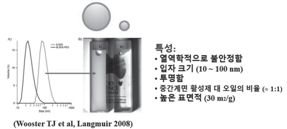
Fig. 4. Physicochemical properties of nanoemulsion (Wooster et al., 2008).
