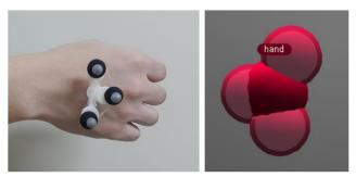
Fig. 3. Three retroreflective markers were attached to a 3Dprinted sculpture (left). Then, their center point was calculated (right).
