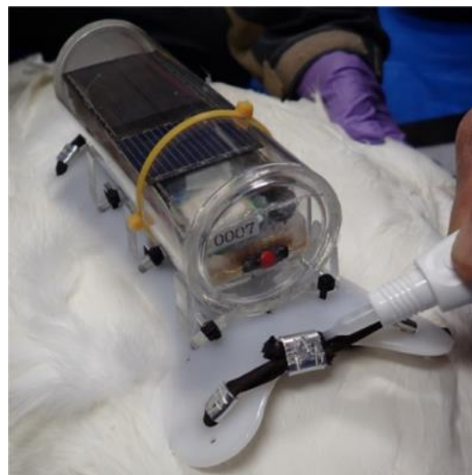
Fig. 11. Packet transceiver on the back of a swan (courtesy of Yamashina Institute for Ornithology)
