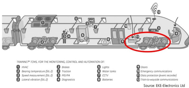
<Figure 4> System Architecture of Driving Part and Related Sensors
