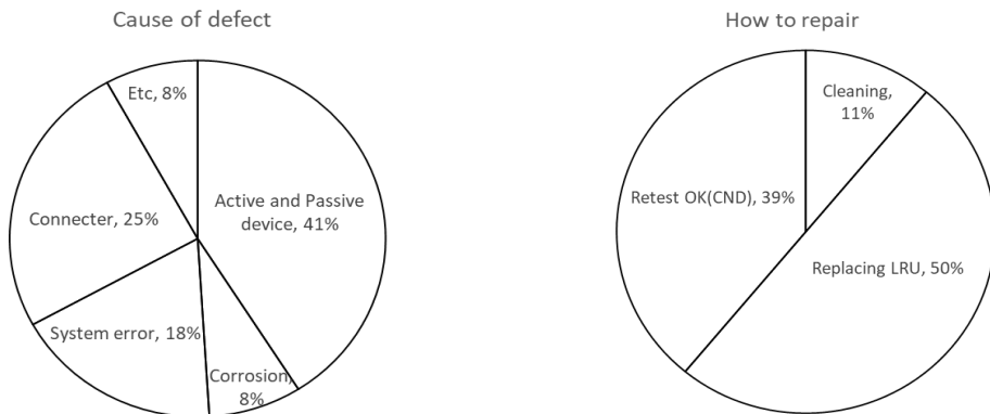
Fig. 3 Defect and repair method of RADAR system
