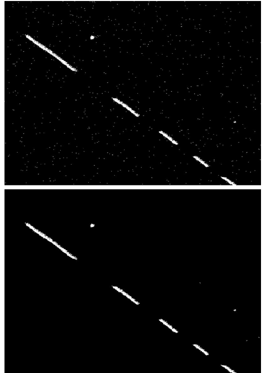
Fig. 5. The foreground image (top) and the foreground image that single pixels are removed (bottom)
