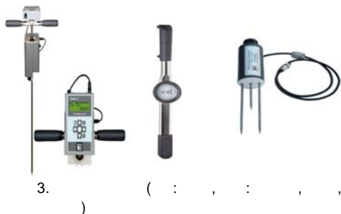
3. Fig. 3. Photos of soil environment sensors (left : soil strength, right : moisture content, temperature, and EC)
