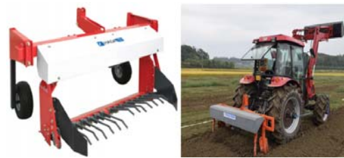
4. Fig. 4. Photos of underground crop harvester (left) and its traction operation attached to agricultural tractor (right)
