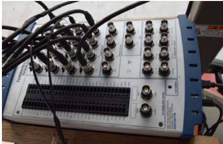
2. Fig. 2. Data acquisition system installed in the tractor
