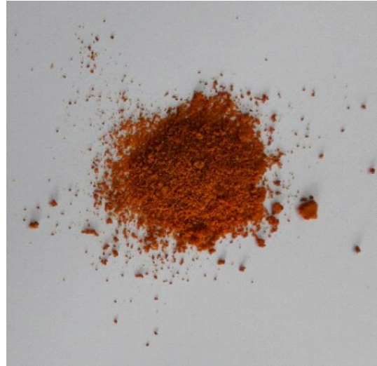
Fig. 10. A photograph showing the encrusted deposits on the low temperature part of the quartz tube after the experiment using CO-Cl 2 gas mixture.
