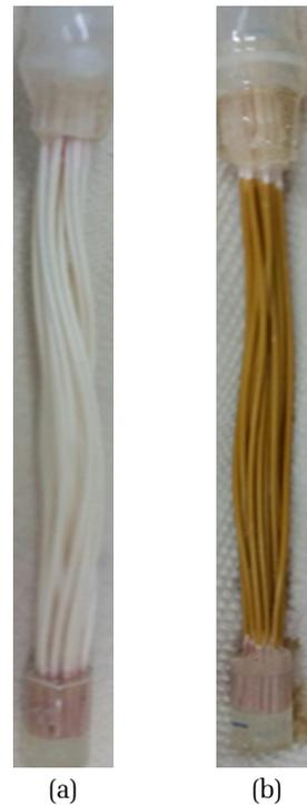
**Fig. 9.** Fouled membrane modules in the continuous experiment for (a) membrane filtration without any oxidant injection and (b) membrane filtration with multiple injection of  $\text{KMnO}_4$  and  $\text{NaOCl}$ .
