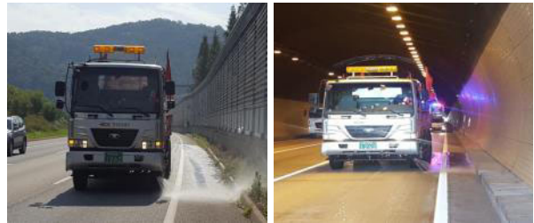
Fig. 4 Earthwork Washing(Left) and Tunnel Washing(Right)
