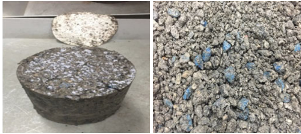
(a) Specimens (b) Mixture Fig. 7 Mixing Paint Aggregate
