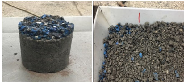
(a) Specimens (b) Mixture Fig. 6 Chipping Paint Aggregate
