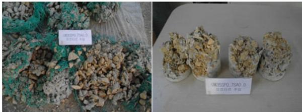
Fig. 17 Paste Infiltration of Pour-over Method and Core Inside
