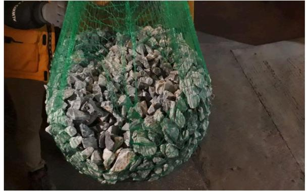
Fig. 16 PE Netting (25mm×25mm)
