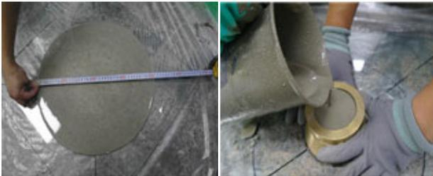
Fig. 10 Miniflow Test of Cement Paste for Gravel Coating
