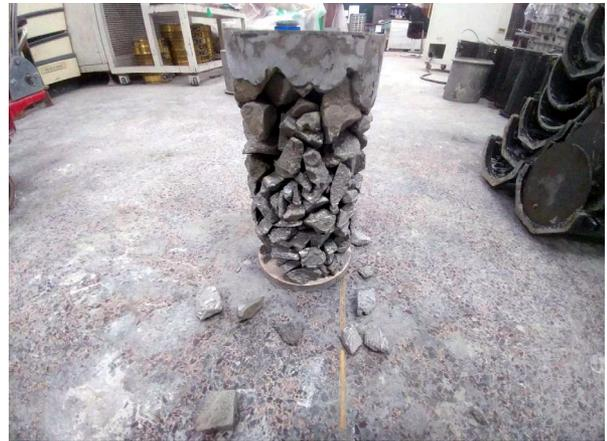
Fig. 11 Insufficiently Coated Gravel
