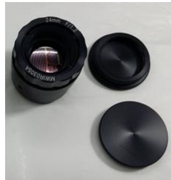
Fig. 6. External view of the assembled barrel with the optimized MWIR imaging lens system
