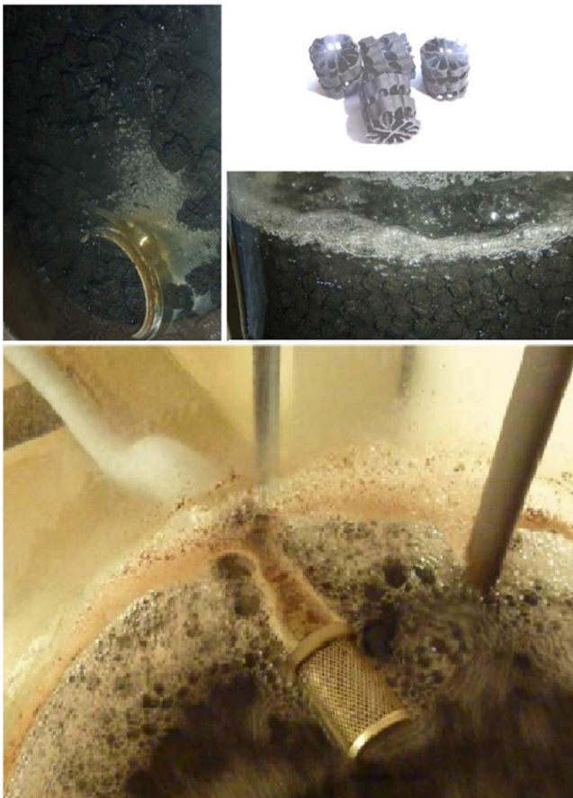
Fig. 3. Meteor 360 media, pilot effluent pipe with media retaining screen.
