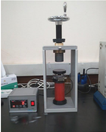
Figure 6. Compressive strength measuring device.
