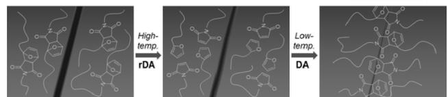
**Figure 4.** Thermally reversible self-healing polymer network based on Diels-Alder chemistry.
