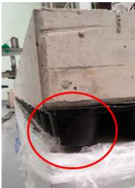
Figure 12. Deformation due to curling
