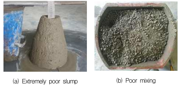
Figure 6. Typical problems of lightweight concrete with low unit water content
