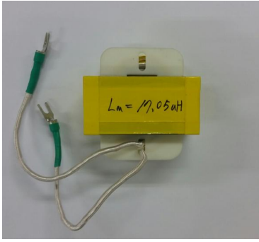
Fig. 11. Resonant inductor used in the proposed converter.
