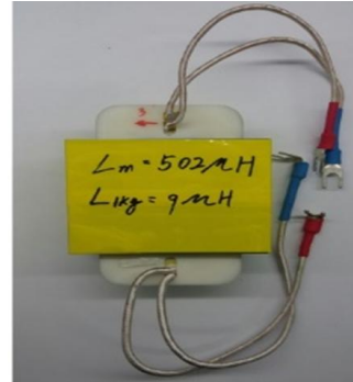
Fig. 10. Transformer used in the proposed converter.
