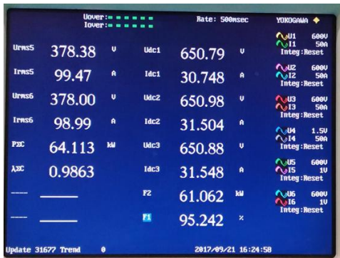
Fig. 20. Measured efficiency of 60kW rapid EV charger with the proposed converter.
