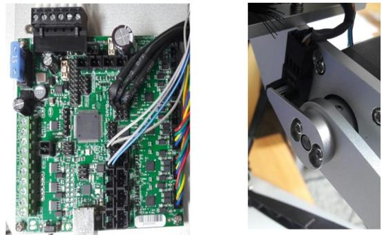
Fig. 8 Motion Controller and Photo Sensor Assembly
