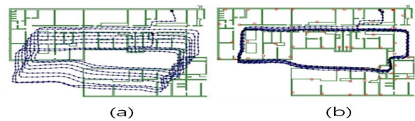
[Figure 10] Accumulated error in the PDR technique (a) and calibration results (b)
