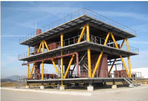
Fig. 4 A Hypothetical topside model for gas explosion tests
