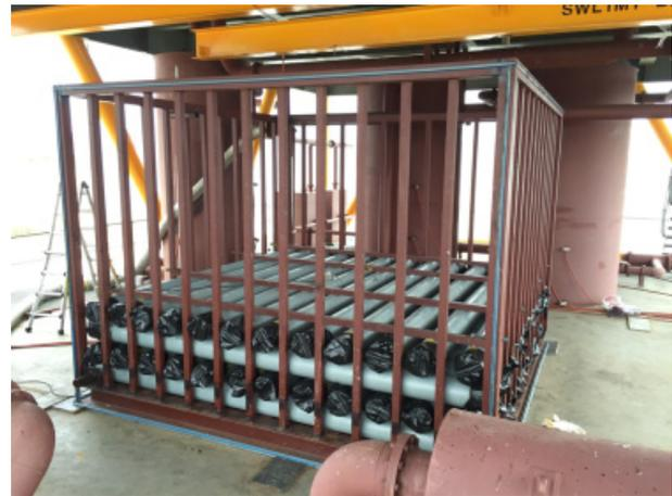
Fig. 9 Layout of the dummy pipes with 12 pipes x 4 rows (Case V)
