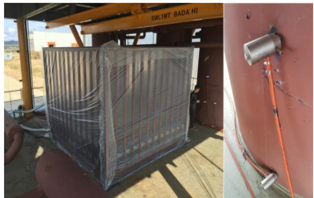
Fig. 6 A test jig for the modeling of gas clouds and installations of pressure sensors
