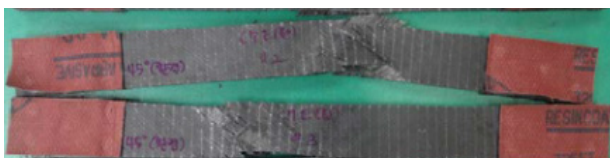
Fig. 18 Picture of damaged CFRP shear specimen
