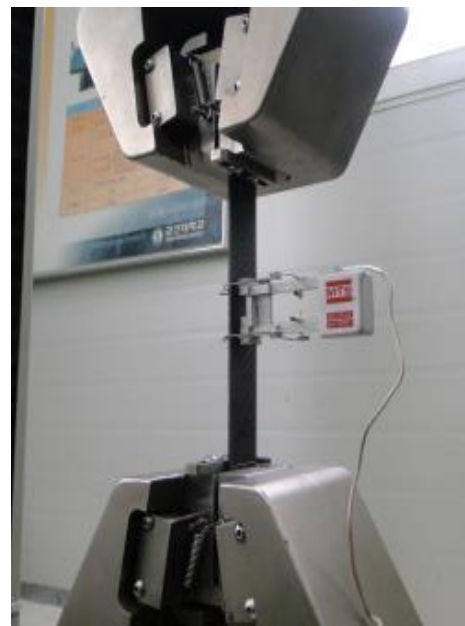
Fig. 15 In-plane shear test of CFRP test specimen
