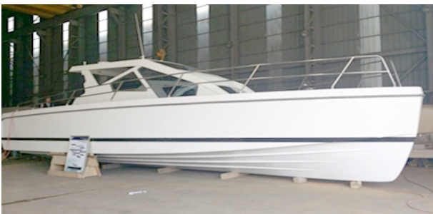
Fig. 2 Marine leisure boat built in CFRP
