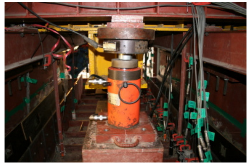
(b) Loading on the plate with hydraulic cylinders
