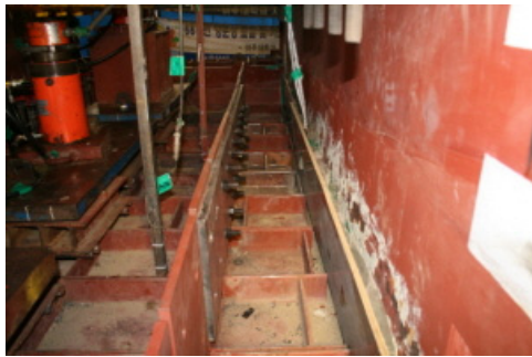
(a) Installation of loading plate
