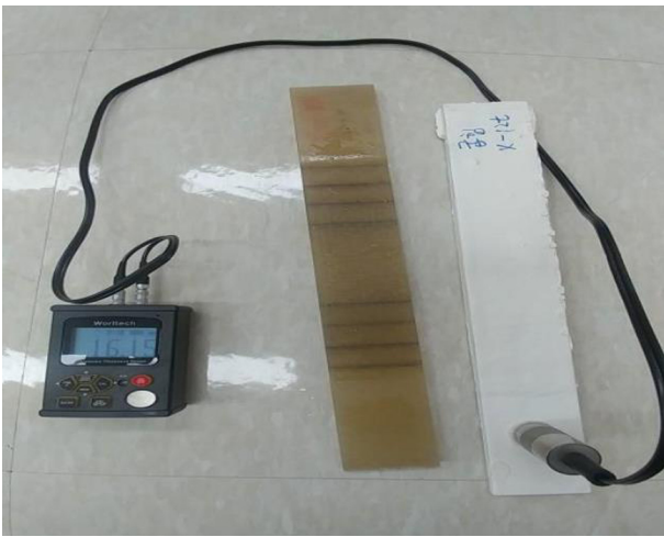
Fig. 5. Measuring the thickness of the gel coating specimen.
