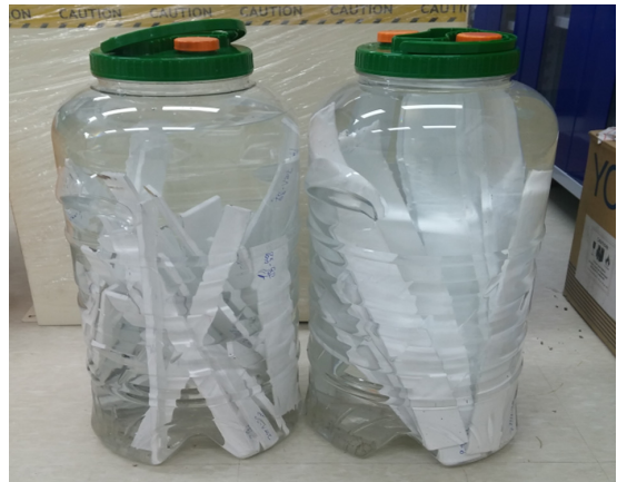
Fig. 4. Sea water storage for coated test specimen.
