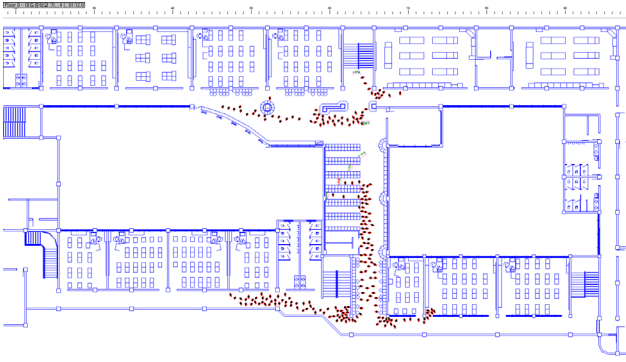
Figure 3. Flow diagram at 60 seconds after start of movement by SIMULEX program 12)
