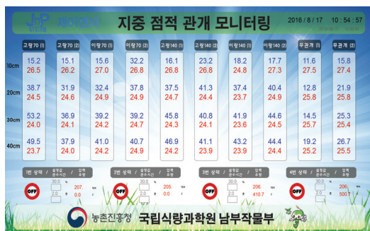
Fig. 1 Graphic user application for monitoring soil moisture and temperature in subsurface drip irrigation
